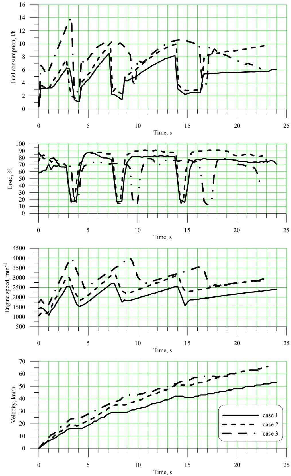
**Fig. 6. Comparison display of the specific parameters by different driving cases driving uphill along the road grade of 4.29 %**
