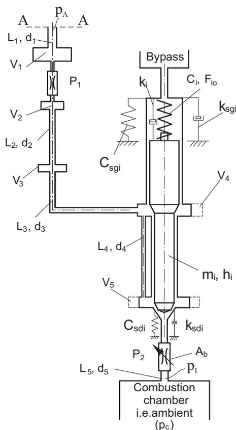
**Fig. 1. Physical model of fuel injection system with special attention to the injector modelling**
