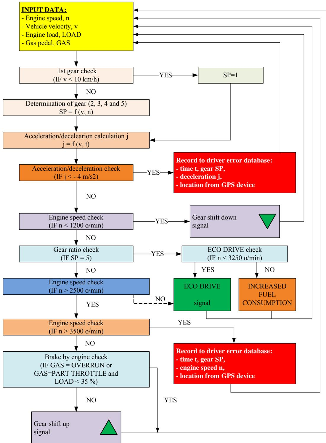
**Fig.6. Algorithm to achieve the optimal drive and optimal fuel consumption**
