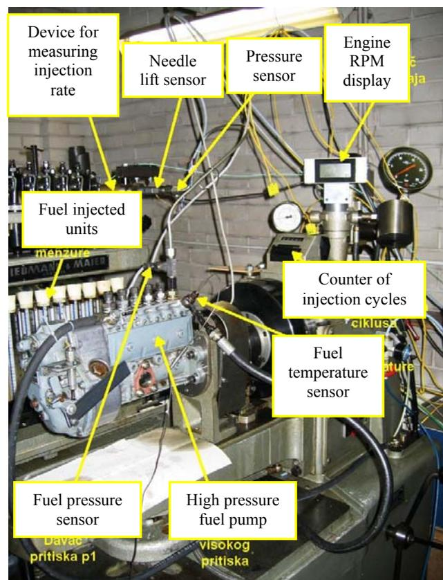
**Fig. 2. Fuel injection system with marked locations of measurement devices**
