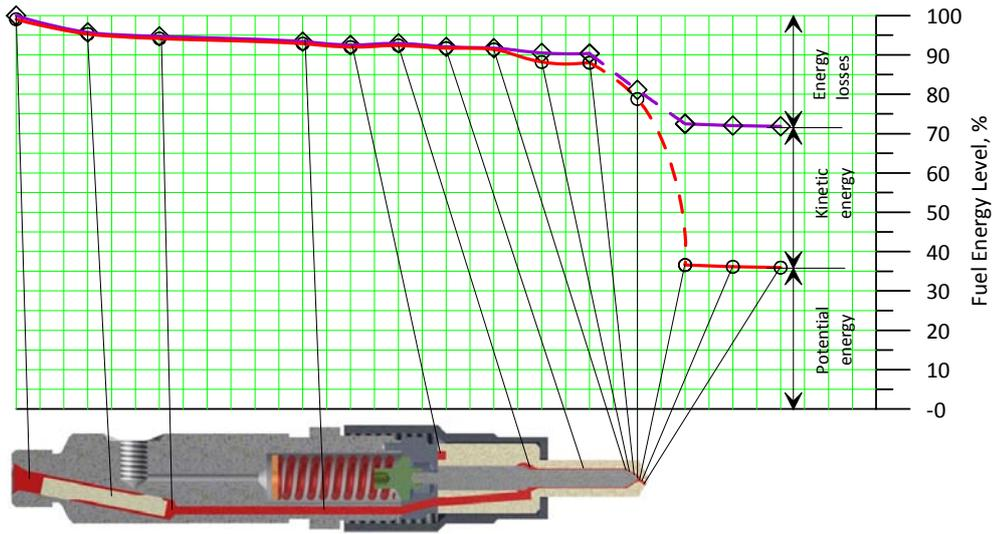
**Fig 3. Transformation of fuel energy along the injector at maximum value of fuel pressure at the end of high pressure pipe and at the maximum of high pressure pump speed of 1100 rpm**
