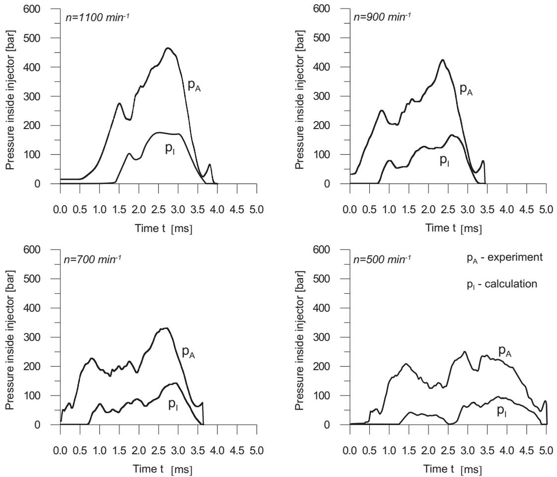
**Fig 4. Trend of measured fuel pressure ( $p_A$ ) and calculated fuel pressure ( $p_I$ ) for different engine speeds oh high pressure pump**
