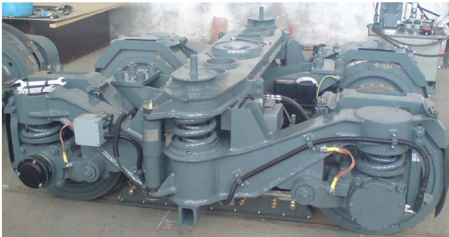
Figure 3. The bogie at the extremities in body “C” urban rail vehicle.
