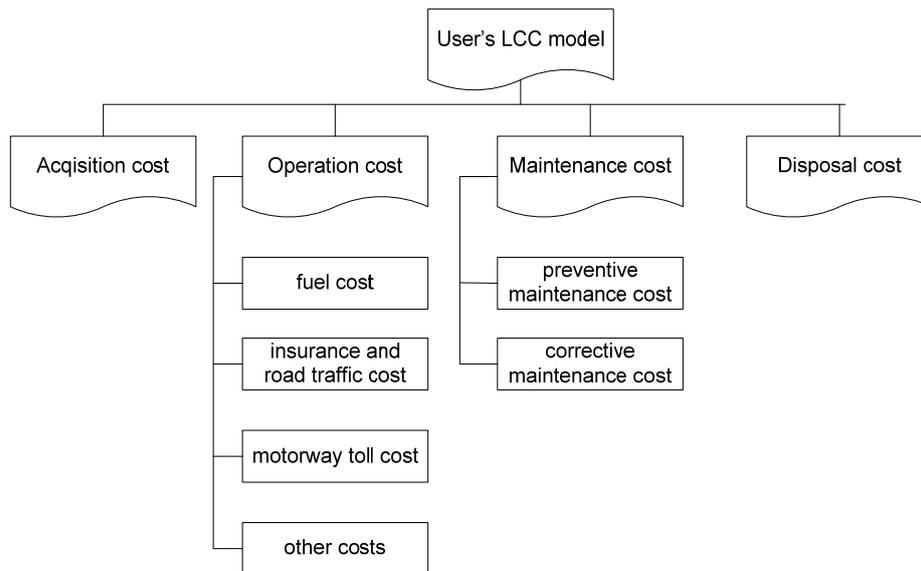
**Fig 1: LCC model of a vehicle**
