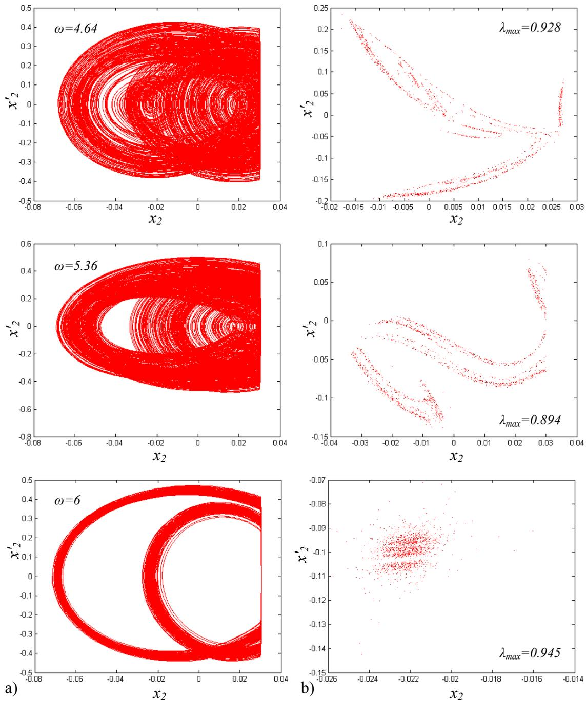
**Fig.7. Projection of the system attractor (a) and Poincare cross section (b) for  $\omega=4.64, \omega=5.36$  and  $\omega=6 \text{ rad/s}$**
