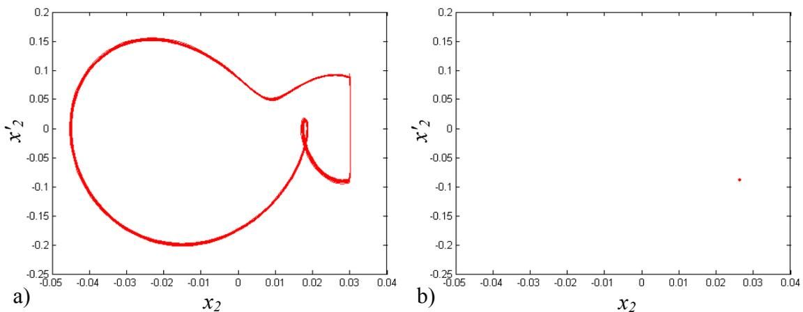
**Fig.5. Projection of the system attractor (a) and Poincare cross section (b) for  $\omega=3.64$  rad/s**
