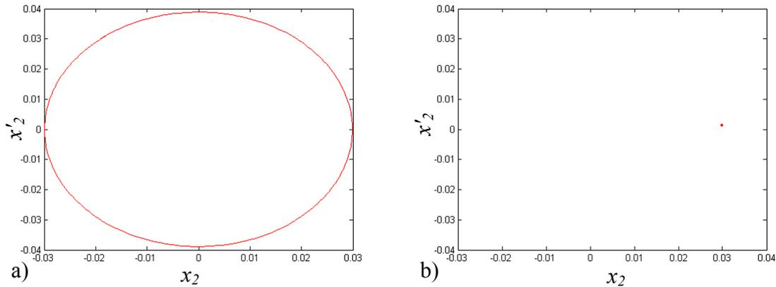
**Fig.4. Projection of the system attractor (a) and Poincare cross section (b) for  $\omega=1.3$  rad/s**
