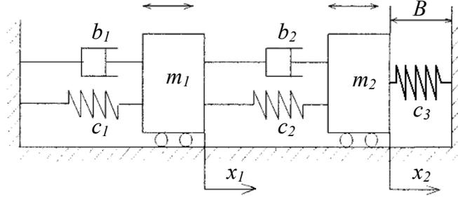
**Fig.1. Model of vibro impact system with two degrees of freedom**
