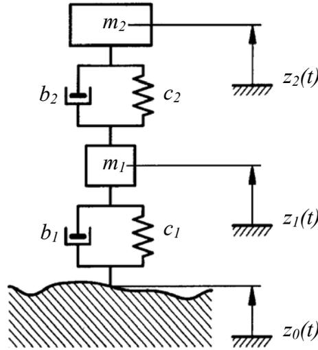
Fig.8. Quarter nonlinear vehicle dynamical model with two degrees of freedom
