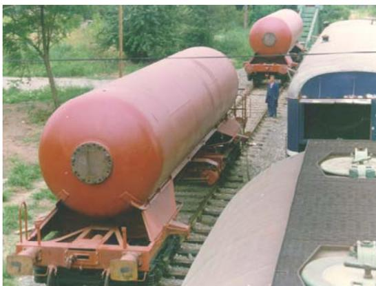
**Fig.2. Test polygon for wagons impact research**
