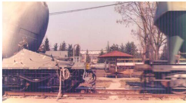
**Fig.4. Two wagons impact on test polygon**
