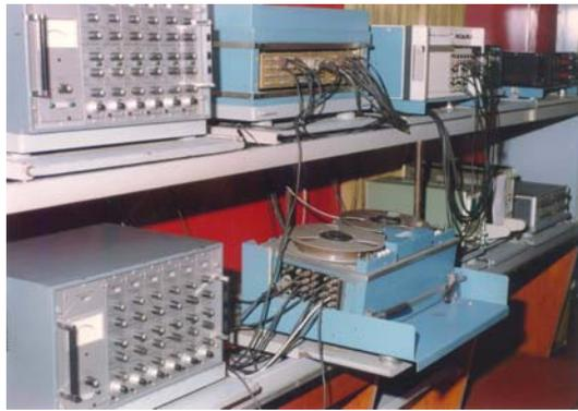
**Fig.3. Measurement equipment for wagons impact research**
