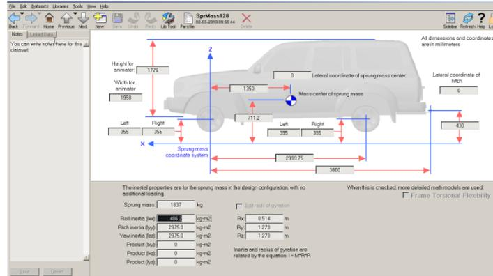
Fig. 6. Geometrical parameters of the vehicle.
