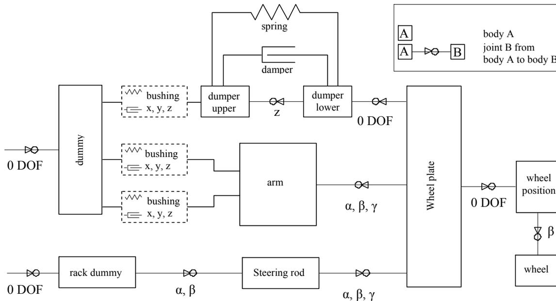
Fig.2. Algorithm of the McPherson front wheel suspension with elastokinematics.
