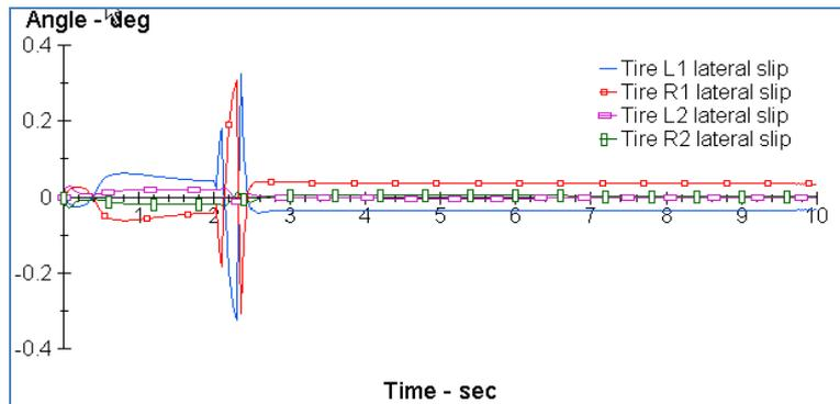
Fig. 8. Slipping angle of the tires.
