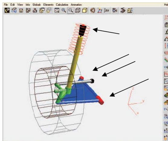
Fig.3. Graphic representation of the multibody model of the McPherson strut
