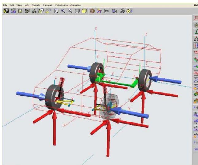
*Fig. 1. Graphic representation of a multibody model of a middle-class vehicle.*
